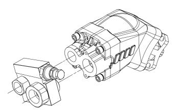
The fitment of the relief valve assembly onto the pump is **symmetric**, thus it is possible to **rotate it by 180°** just to avoid any interferences.
